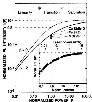
Fig. 1. Normalized luminescence intensity  $I$  as a function of normalized laser power  $P$  with  $\beta = 0$  and 2. The experimental data points ( $\times$ ) at  $P = 1$  are given for three samples. The inset shows the Er PL intensity versus excitation power with the solid line as the best fit to Eq. (6) for sample Cz-Si:Er,O.
