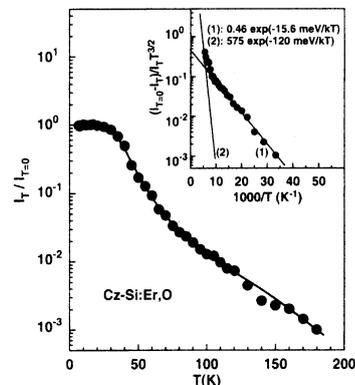
Fig. 2. PL intensity as a function of sample temperature normalized to the yield at low temperature. The solid line is the fit with Eq. (8). The inset plots  $(I_{T=0} - I_T)/I_T T^{3/2}$  as a function of reciprocal temperature illustrating the analysis based on Eq. (9) for sample Cz-Si:Er,O.
